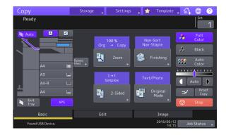
Copying and printing are set to default to **mono and duplex** – if you want single sided or colour please ensure you change the settings before pressing print. To copy on a different paper type use the bypass tray then select the tray you are using on the screen.
