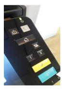
Tip: At any time you can go to the user information screen by pressing the number '2' button, or to the Copy screen by pressing the number '1' button.
